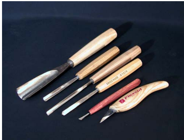
Hand carving tools large, medium, and small gouge, v-tool, angled blade, knife
